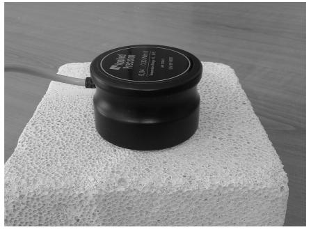
Fig. 1. Surface probe in material G measurement
