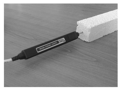
Fig. 2. Needle probe in material F measurement
